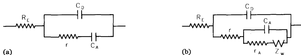
Fig. 1. Equivalent circuits for hydrogen adsorption on a palladium electrode in 0.1 M NaOH solution: (a) simplified circuit; (b) the circuit accommodated to the experimental data.
